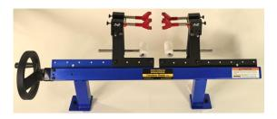
The **Crossbow Master Plus** is designed to cover the needs of pressing crossbows. It allows the bow technician to be close to the hand wheel when working on a crossbow while operating the bow press.
